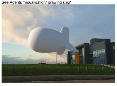
1.1.1 The development involves an inflated helium airship/blimp shaped balloon attached to a winch, which would carry up to 30 passengers in a gondola suspended beneath. It would be raised up to a maximum height of 120 metres on an 8 minute ride (4 minutes to rise and 4 minutes to descend) with the objective of viewing the surrounding area and Rhyl Coastline from a height. See plans snip below\*
